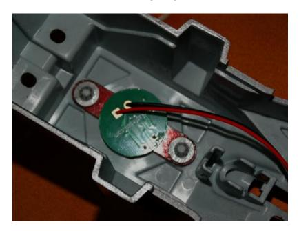
6. Remove the current wedge 555 bulb for both the left and right-side cannons. Take the wedge type female wire harness (as shown below) and insert into the wedge 555 bulb socket.
