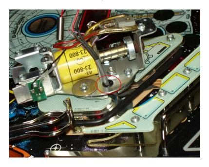
7. Insert **female** end of the twelve-inch cable assembly through the available holes from under the playfield and then through the hole in the cannon assembly as shown below.
