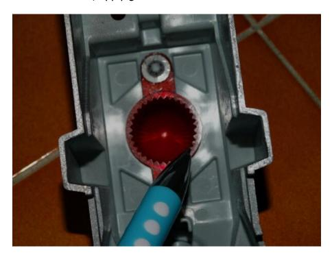
It should look like this after gluing the Red LED Oscillator in place.
